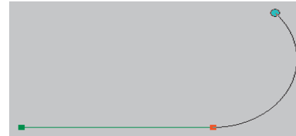
Once a line segment has been sketched, the Tangent Curve tool will draw a circular arc off of the previous line segment.
